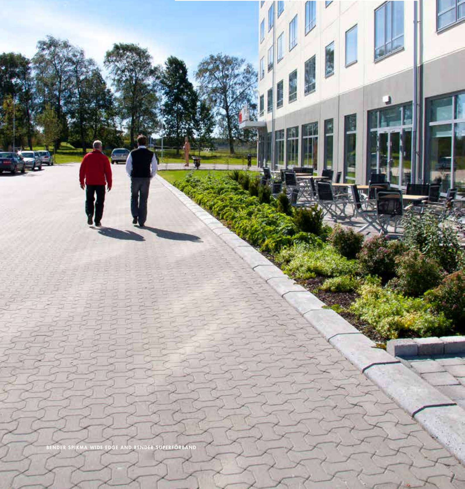
BENDER SPIKMA WIDE EDGE AND BENDER FLAT SLABS 350X170 MM
