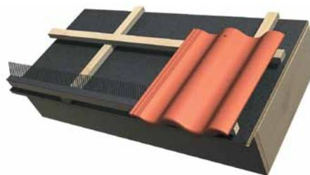
**Figure 14.** The birdstop is attached to the eaves. This prevents birds from nesting under the tiles. There are different kinds of birdstop – ventilating and non-ventilating.
