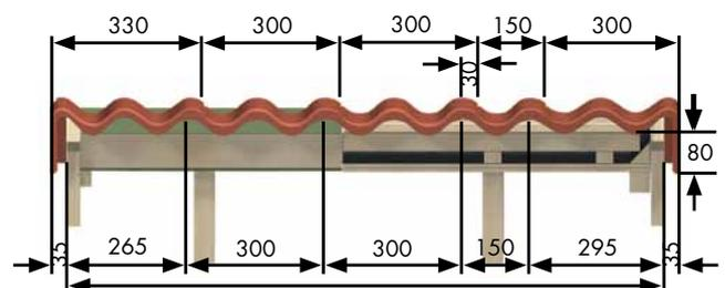
**Figure 9.** Calculate the gables. Get the exact measurement on our homepage, [www.benders.se](http://www.benders.se).
