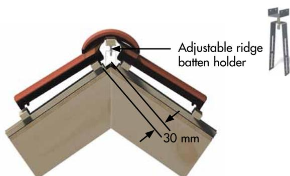
**Figure 5.** The counter battens are omitted entirely when use of roof board.
