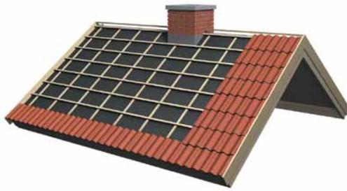
**Figure 10.** Construct from right to left and start by installing the entire lower row (=row closest to the eaves). Start from the right hand side and apply two to three tiles in a row all the way up to the ridge. Make sure that the rows are straight.
