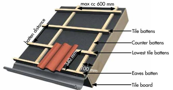
**Figure 2.** The batten distance is measured from top edge to top edge. Note that the distance from the eaves batten edge to the eaves battens top edge should not exceed 340 mm. Also note that the eaves batten should be 20 mm wider than the rest of the tile battens, as the lower tiles do not rest on other tiles (does not apply on ventilating birdstops).
