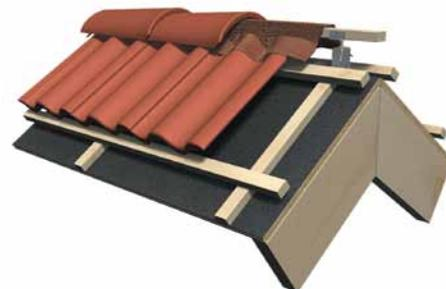
**Figure 3.** The distance between the ridge batten and the upper tile batten should be around 30 mm. Make sure that the ridge tiles covers the nail holes on the upper tiles.
