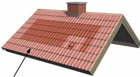
**Figure 11.** Nail all the highlighted tiles.
