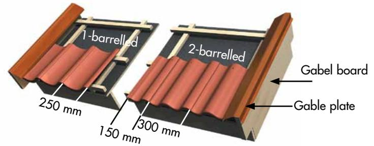
**Figure 6.** Calculate the roofs width in tiles. Note that the last tile, closest to the gable, should have a width of 300 mm.
