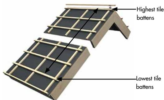
**Figure 4.** Use the distance between the upper and lower battens to calculate the correct batten distances.
