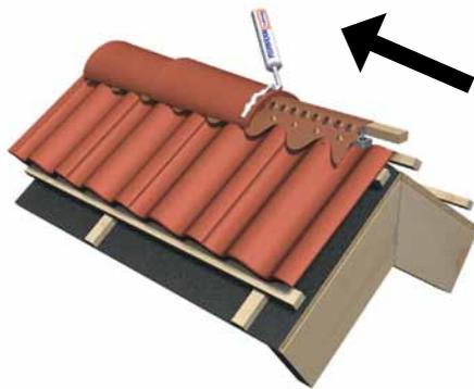
**Figure 12.** Insulation of a paperboard underlay with closed ridge. Benders Ventiridge is applied and attached in order to protect the ridge from precipitation. It also ventilates, this prevents the roof from rotting.
