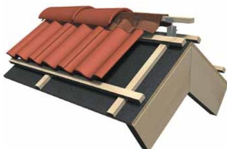
**Figure 13.** Benders ridge roll is easy to install. Attach the ridge roll to the ridge batten – by nailing or stapling. Remove the protective tape on the bottom of the roll and press to form the roll after the tiles.
