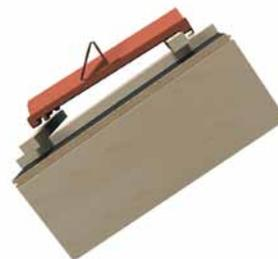
**Figure 16.** In order to prevent damages to the valleys caused by sliding snow, install snow hooks. Snow hooks are very easy to install. Use about 3-4 per m<sup>2</sup>.
