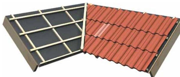
**Figure 15.** By valleys, use half tiles to prevent the usage of too small pieces of tiles that can be difficult to attach and nail (only apply to 2-barrelled tiles). The half tile is highlighted in the figure. Mark the tiles on the roof – cut them on the ground – rinse the tiles with water directly after cutting!
