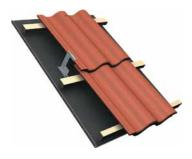
**Figure 8.** The clip is installed in a way that locks both tiles to the batten.
