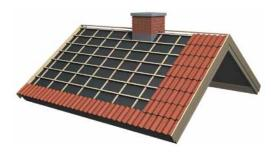
**Figure 10.** Construct from right to left and start by installing the entire lower row (=row closest to the eaves). Start from the right hand side and apply two to three tiles in a row all the way up to the ridge. Make sure that the rows are straight.
