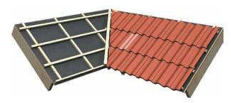
**Figure 15.** By valleys, use half tiles to prevent the usage of too small pieces of tiles that can be difficult to attach and nail (only apply to 2-barrelled tiles). The half tile is highlighted in the figure. Mark the tiles on the roof – cut them on the ground – rinse the tiles with water directly after cutting!
