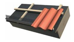
**Figure 14.** The birdstop is attached to the eaves. This prevents birds from nesting under the tiles. There are different kinds of birdstop – ventililating and non-ventilating.
