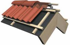
**Figure 13.** Benders ridge roll is easy to install. Attach the ridge roll to the ridge batten – by nailing or stapling. Remove the protective tape on the bottom of the roll and press to form the roll after the tiles.
