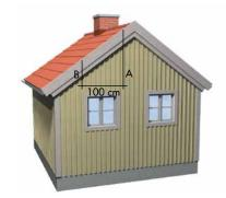
**Figure 1.** Subtract measured number (B) from measured number (A) to get the roof pitch, See table 1.
