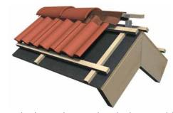
**Figure 3.** The distance between the ridge batten and the upper tile batten should be around 30 mm. Make sure that the ridge tiles covers the nail holes on the upper tiles.
